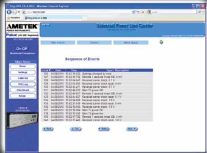
SOEs - View and download the up to 4096 SOEs available in the unit.
