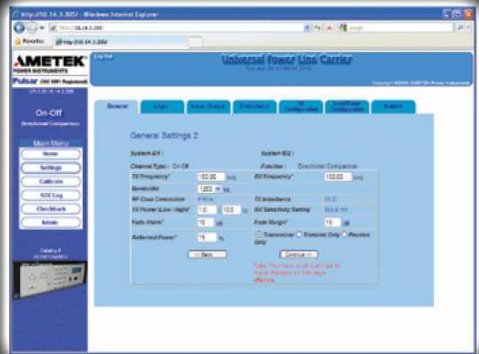
General Settings Page - Set the frequencies, transmit power, receiver margin, etc. A red "Changes Pending" bar appears at the top of the screen when changes are made.
