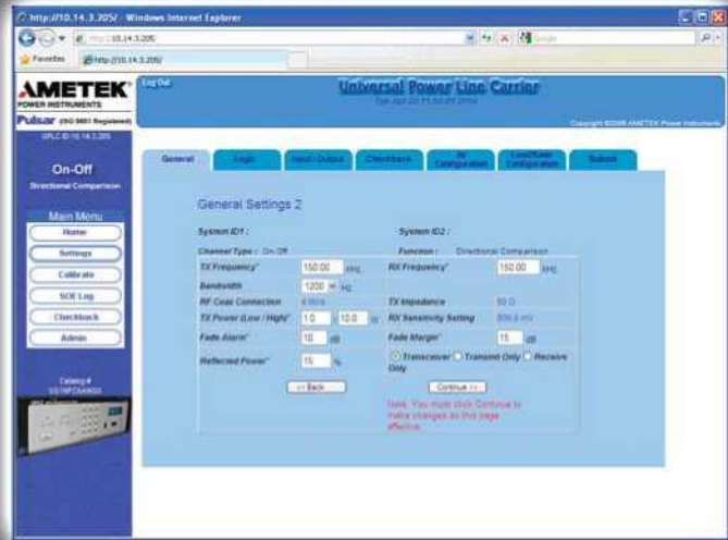
General Settings Page - Set the frequencies, transmit power, receiver margin, etc. A red "Changes Pending" bar appears at the top of the screen when changes are made.
