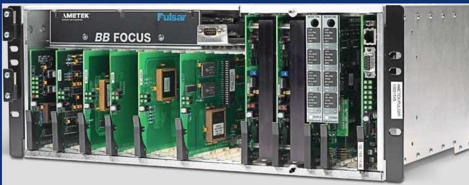
Front view of the BB FOCUS (left) with cover removed, revealing the location of DS0 Channel Cards (lower right), and Common Modules (lower left), with the optional integrated Ethernet switch location above the DS0 Channel Cards section.
